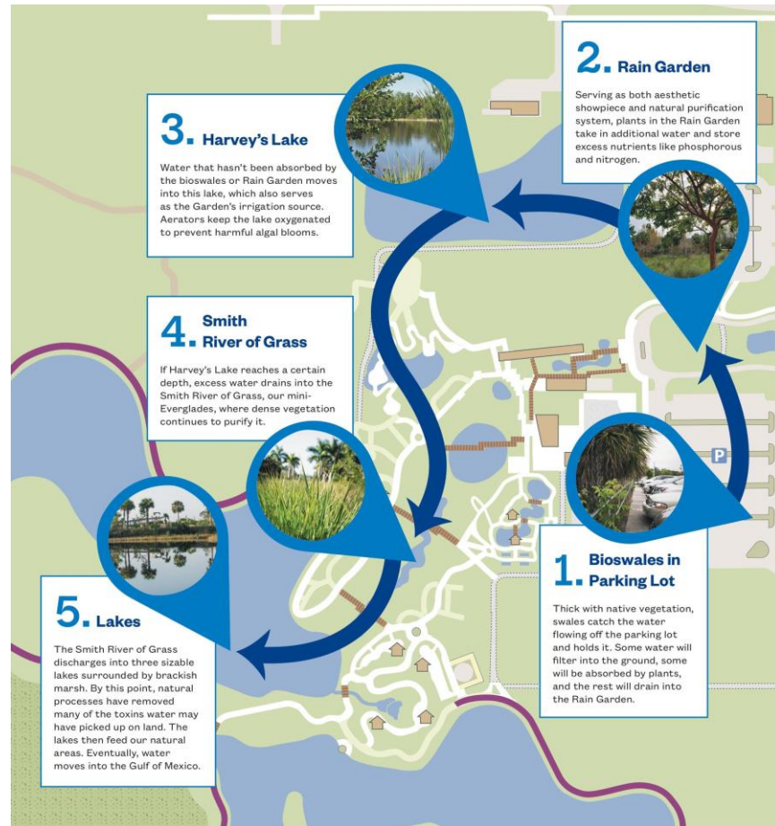
Figure 2. Overall stormwater system and individual components at Naples Botanical Garden in Naples, FL, USA.
