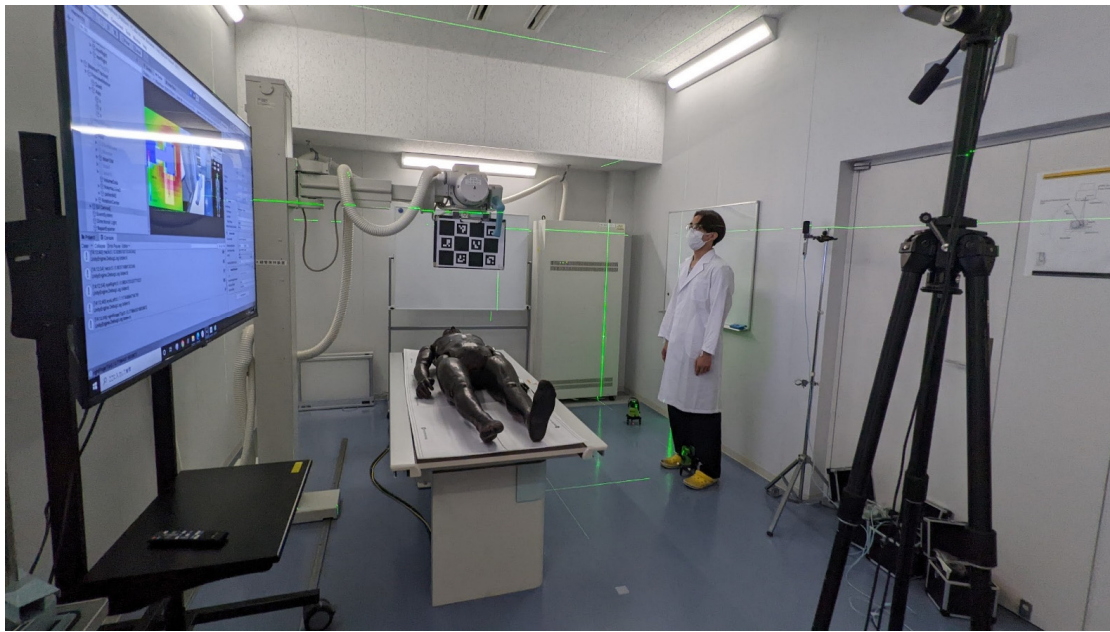
Figure 6. Arrangement of equipment in the X-ray room when using the system.
