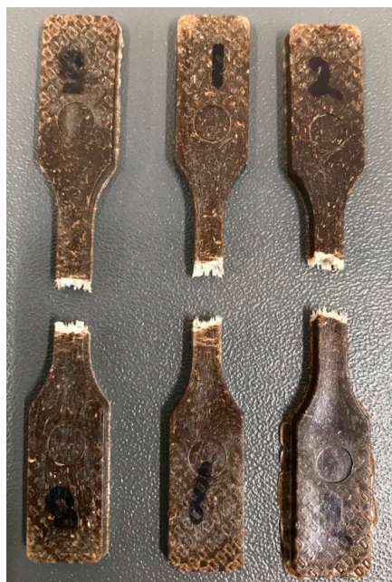
Figure 3. Tensile-broken specimens corresponding to PP/WF-5901, PP/WF-5951, and PP/WF-0218 composites.
