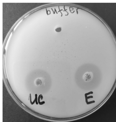
Figure 2. Clear halos were observed in agar plates containing 0.1% PCL (MW 14,000) when 50 \mu L containing 145 U of UC (ultraconcentrate) or E (pure enzyme) were incubated in the holes at 55 ^{\circ} C for 24 h. Buffer was used as a control.
