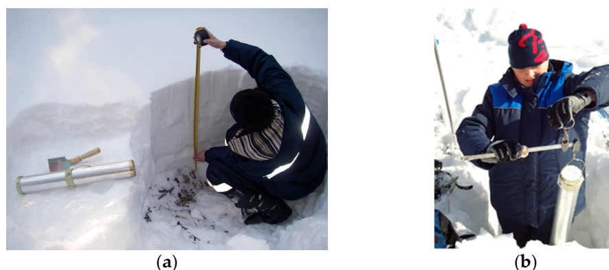
Figure 9. Snow sampling procedure: (a) measuring the height of the snow cover; (b) weighing the snow.
