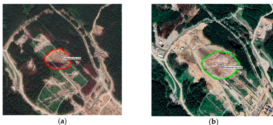
Figure 8. Solikamsk-2 potash mine location; the background image was obtained from Google Earth: (a) August, 2016; the red line—collapse of the Solikamsk-2 potash mine; (b) August, 2022; the green line—the eliminated collapse sinkhole.
