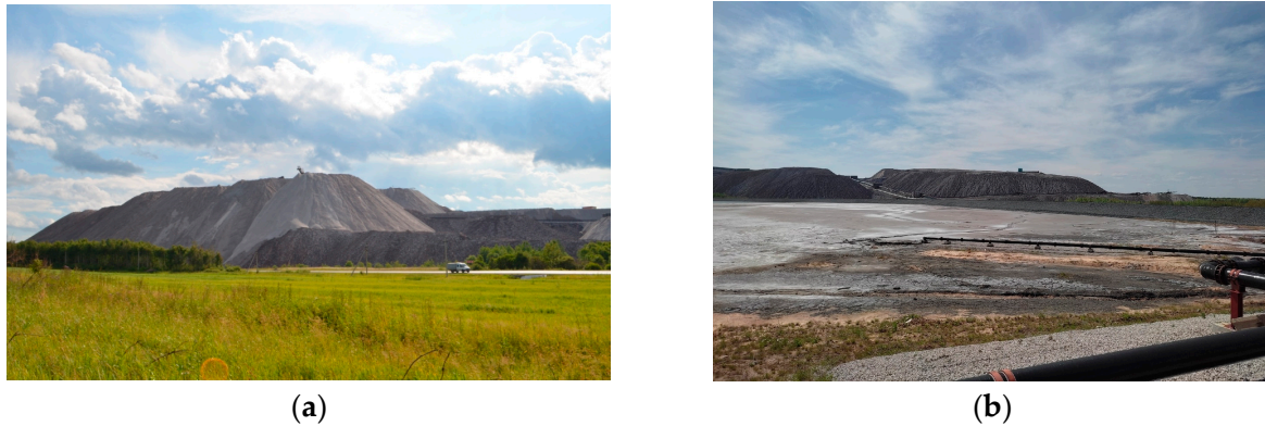
Figure 4. Potash ore processing waste disposal facilities on the Verkhnekamskoe deposit's territory: (a) potash tailings pile; (b) potash tailings slurry.
