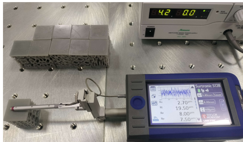
Figure 5. Setup for roughness determination using Surtronic S128.
