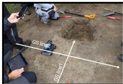
Figure 18. GS8000 transect lines surveyed after the removal of surface vegetation and before the completion of excavation of Feature 1. Wrocław, Poland, police compound. 21 September 2021 (photo by F.C.).
