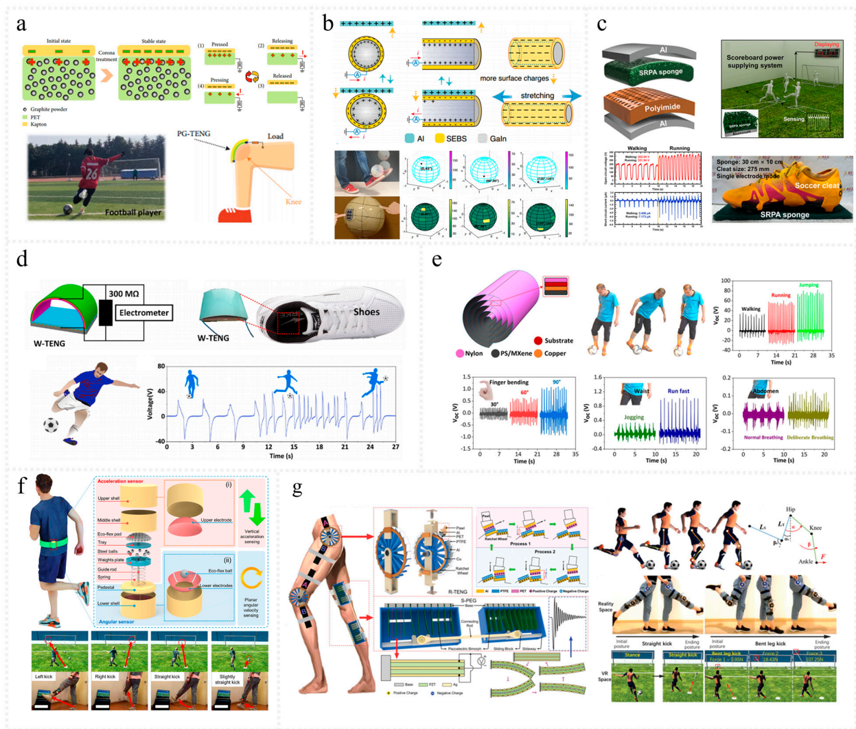
Figure 5. Application of TENG-based sensors in football. (a) Diagram of the working principle and PG-TENG installed on the human knee [55]. (b) Working mechanism of the ultra-stretchable fiber TENG and conductive fibers on a 3D surface of a football to perform the sensing function of a spherical coordinate [56]. (c) Structure and application of SRPA sponge for the self-powered scoreboard power supplying system. Reprinted with permission from Ref. [57]. Copyright 2021, American Chemical Society. (d) System architecture diagram of self-power football motion monitoring system. Reprinted with permission from Ref. [58]. Copyright 2022. Elsevier. (e) Structural diagram of the PM-TENG and its performance in monitoring different motion postures [59]. (f) Structure of the multidimensional sensor and demonstration of the VR football shooting game [60]. (g) Configuration of the MC-EH-HL system, which consists of two main components, R-TENG and S-PEG, and detailed motion segments of a kicking process with two R-TENGs fixed on the hip and knee joints [61].
