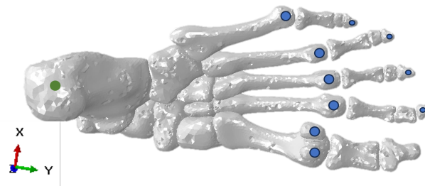
Figure 3. Fixed nodes (green) and displacement constraint (blue) locations for the simulation of the mid-stance of the gait cycle.
