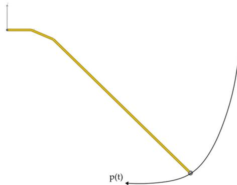
**Figure A1.** The deformation of the PRBM when the position of the tip is specified directly. The gray point moves along a defined path  $p(t)$ . The tip of the PRBM is connected to the point with a spherical joint (6 DOF). This creates a closed kinematic loop and the force-dependent kinematics (FDK) can not solve the system in physically correct way, as seen in the way the beam is bend.
