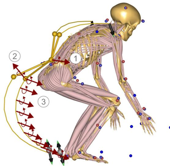
**Figure 6.** Specification of the degrees of freedom that were assigned with a *Stiffness Coefficient* by a force-dependent kinematic (FDK): 1—degrees of freedom of connection to the pelvis in sagittal plane; 2—degrees of freedom of sideway deformation of the PRBM; 3—PRBM degrees of freedom of the lower spring elements. Blue dots are recorded markers from MoCap measurements, red dots are digitally fitted markers.
