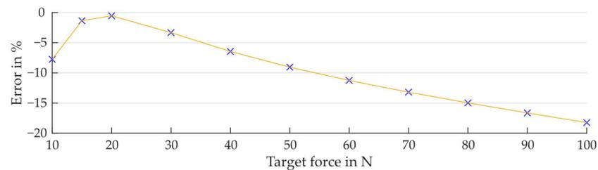
**Figure A3.** Remaining control error of the absolute force of the *Constraint Force*.
