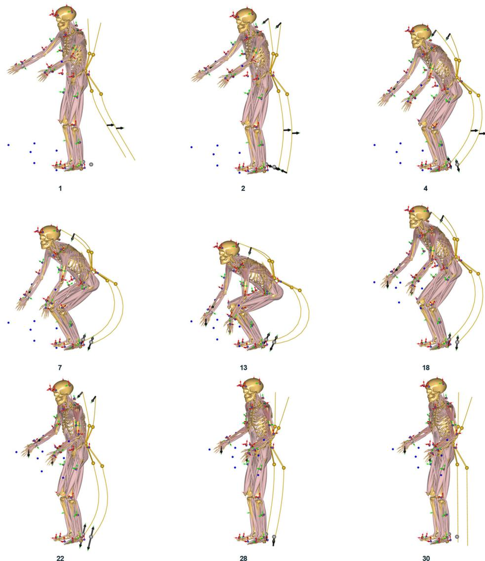
**Figure 8.** Step-by-step illustration of the exoskeleton simulation, the number below the image indicates the respective iteration step. A person lifts a box with the help of the exoskeleton. At the beginning of the simulation, the lower spring elements are deflected by the bending force. At the end of the simulation, the *Constraint Force* is slowly reduced.
