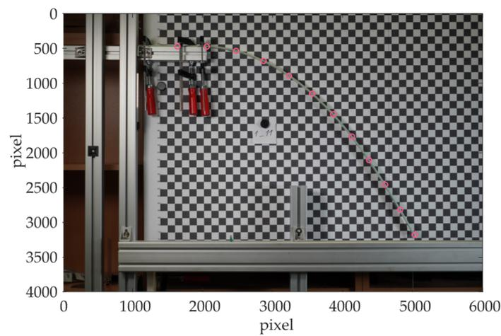
**Figure 2.** Laboratory setup for deforming the flexible beam under defined loads.
