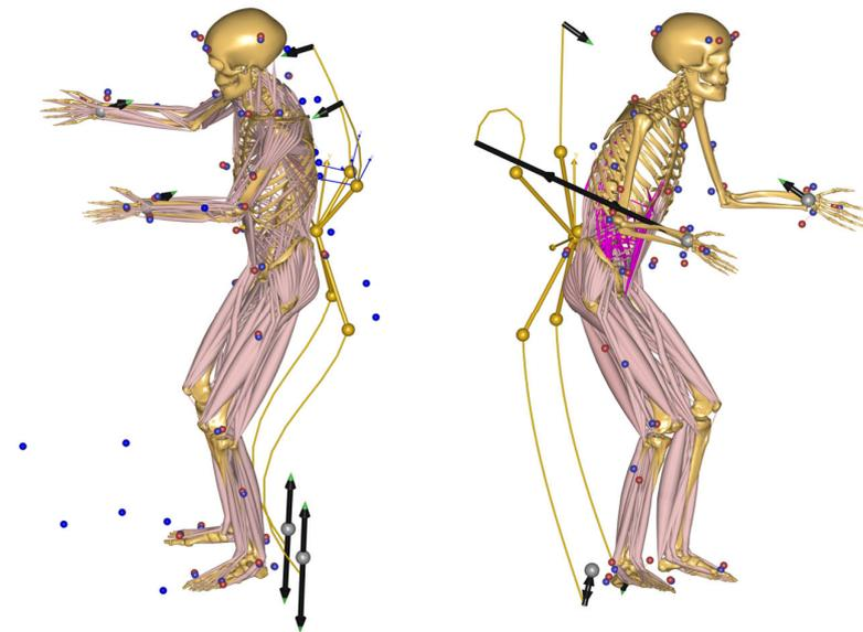
**Figure A5.** Two examples of kinematically unstable positions of the PRBM.
