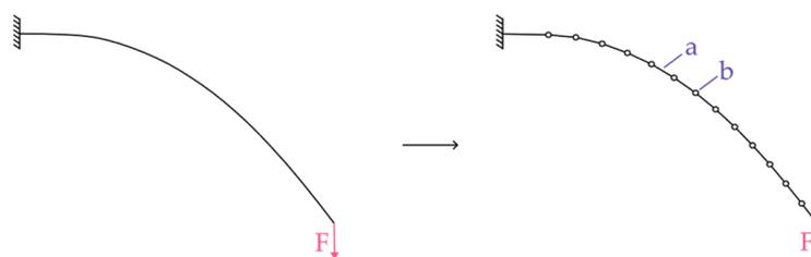
**Figure 1.** The basic idea of a pseudo-rigid-body model (PRBM). A continuous flexible beam is replaced with a chain of rigid segments (a) connected with joints (b). Every joint has a torsion stiffness in the direction of bending.
