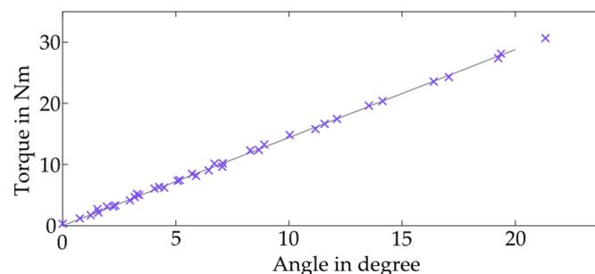
**Figure 3.** The *Stiffness Coefficient* is fitted with the least square method (gray) to the data from three trails under different load condition. The purple data points are each associated with the respective parameters in a joint.
