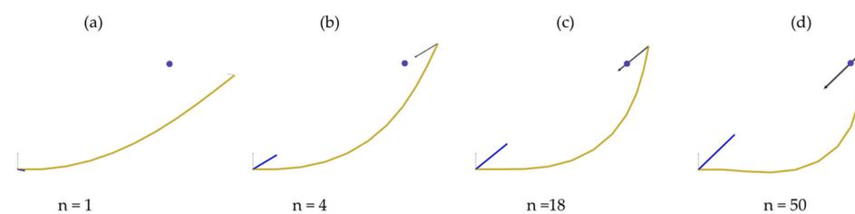
**Figure 4.** Functional principle of the *Constraint Force*. The tip of the PRBM is pulled to the defined point (gray) by the *Constraint Force* (black). The reaction force in the fixed bearing (blue) is also shown. The *Constraint Force* starts to deform at (a) and pulls the PRBM closer and closer to the target point in the course of (b–d). The iteration step of the simulation is indicated below the image in each case.
