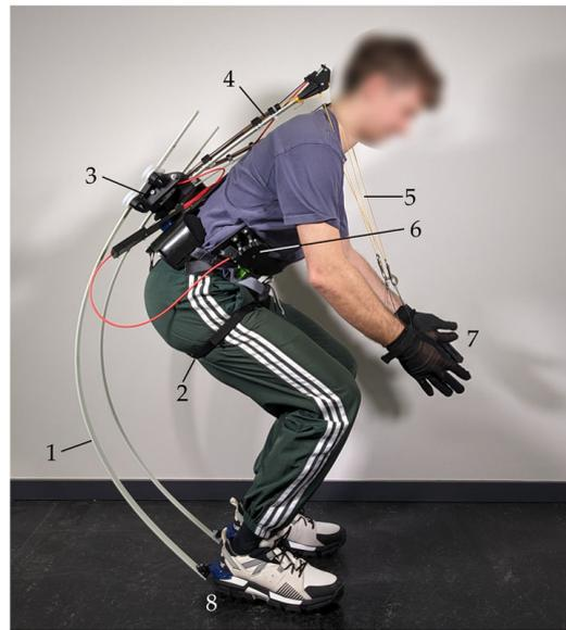
**Figure 5.** Overview of the components of the exoskeleton prototype: 1—lower spring elements; 2—leg straps; 3—back attachment; 4—upper spring elements; 5—strings; 6—actuation lever; 7—gloves; 8—foot attachment.
