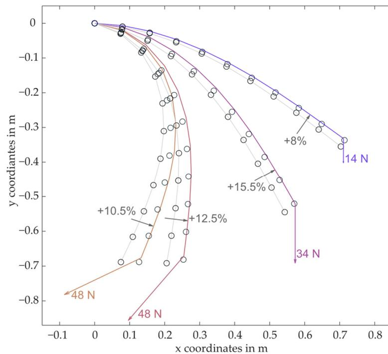
**Figure 7.** Comparison of the measured deformation of a beam in the lab (colored line) with the simulation of the deformation using PRBM (gray line) under four different loads. The black circles represent the joint between the rigid segments of the PRBM.
