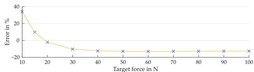
**Figure A4.** Remaining control error of the direction of the *Constraint Force*.
