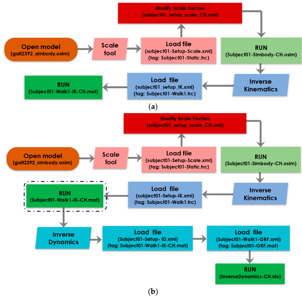
Figure 2. Process flow to run (a) IK for CH model in OpenSim and (b) run ID for CH (CH) model in OpenSim (dotted run block represents the significance of IK compilation before initiating the process of ID).
