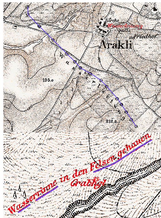
Figure 5. The water conduits were digitized using line geometry. In two different cases, by joining the individual point symbols as they indicate the original/surviving length of the aqueduct or by digitizing the line symbol. The aim was to demonstrate the continuity and the length of the aqueducts.
