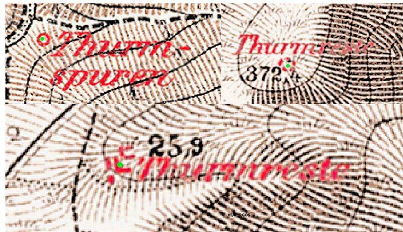
Figure 4. The towers were digitized using point instead of line geometry, avoiding reflecting their floor plan that sometimes appears on the map. In this case, the aim was to preserve the position of the archaeological remains rather than their geometry.
