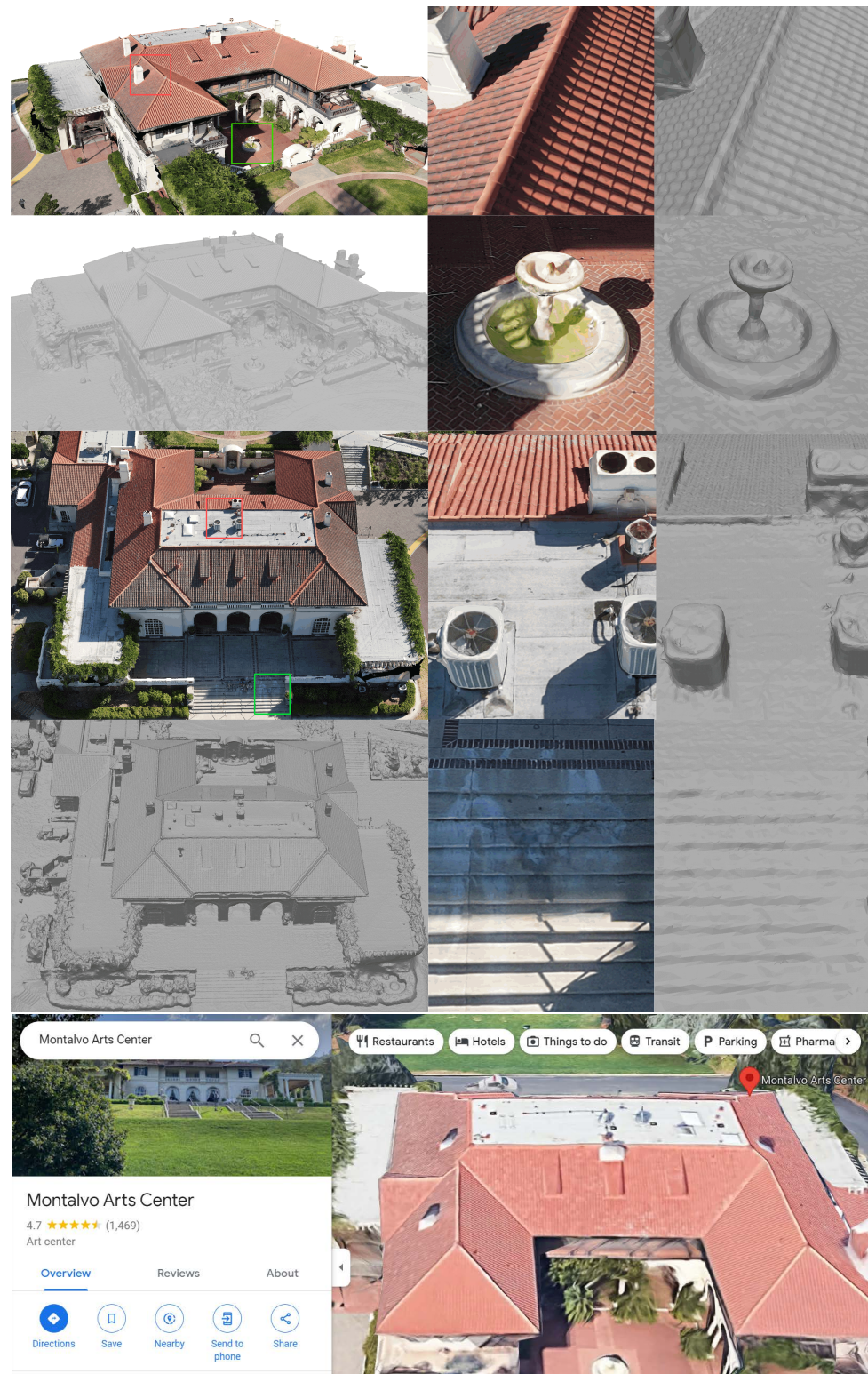
Figure 6. High-Resolution Reconstruction Experiments. We reconstructed the Montalvo Arts Center (Saratoga, CA, USA) using a more recent consumer drone equipped with a 20-megapixel aerial camera (Section 4.2). Rows 1 to 4 show the reconstructed mesh and 3D model with zoom-in views. Note that the zoom level is more than 10 \times . Row 5 shows the same 3D building visualization in Google Maps. The upper and lower enlarged areas are indicated by red and green boxes, respectively. Our results exhibit much-improved quality in both texture and geometry details.
