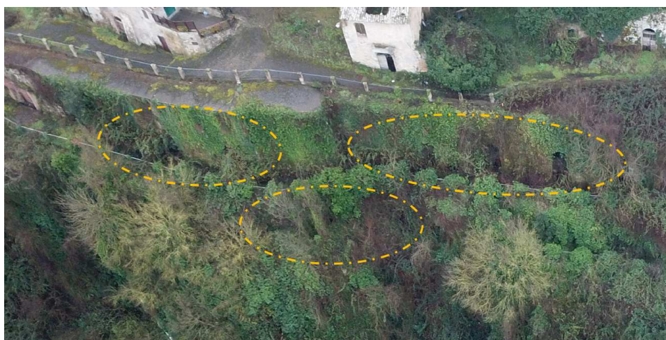
Figure 11. Example of using frontal photos to limit the effects of vegetation. In the orange ovals, some examples of localised entries using frontal photos (inclination of the gimbal 0^{\circ} – 25^{\circ} ).
