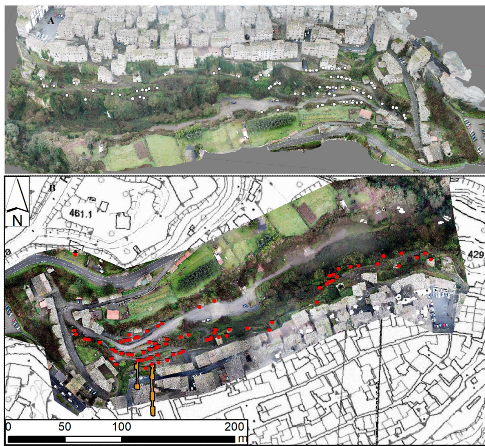
Figure 8. Process of identifying inputs to the model and (A) and transferring the data to the GIS environment ((B) the entrances in red and the floor plans in yellow).
