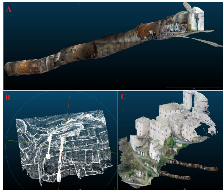
Figure 5. Lidar survey of cavity 2 (A), the final alignment of the 3D cavity models with a detail of the depicted UAV survey to visually appreciate the degree of accuracy (B), 3D model merged in perspective view (C).
