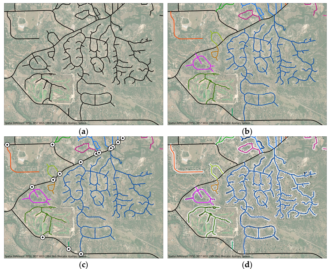
Figure 3. (a) A subsection of the Hays County road network; (b) a subsection of the Hays County road network dissolved and stylized based on the Neighborhoods attribute, such that each neighborhood is represented by a different color and non-neighborhood roads are represented in black; (c) a subsection of the Hays County road network with exits illustrated at the intersections of neighborhood and non-neighborhood roads; (d) neighborhood roads buffered by 100 ft with address points used to estimate the number of households in each neighborhood.
