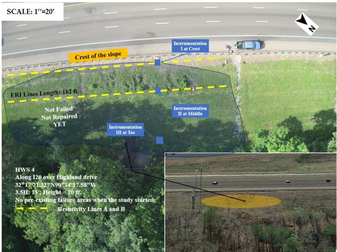
Figure 20. HWS 4 ERI and instrumentation layouts along with its characteristics (drone image-top view) (1' = 1 ft = 0.305 m).
