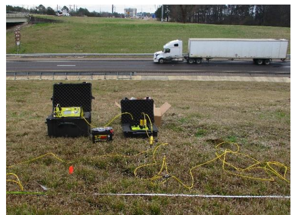
Figure 7. (a) ERI Subsoil current flow profile [25] (b) ERI equipment and field investigation.
