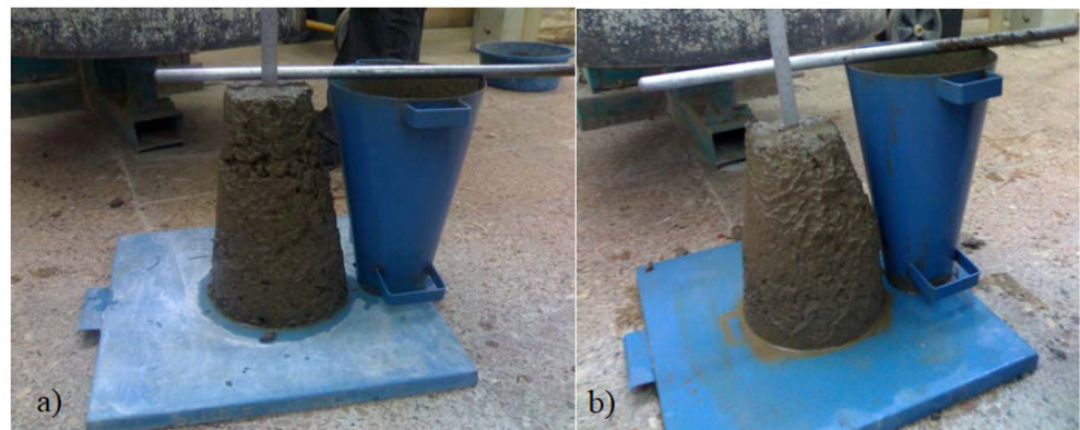
Figure 8. Example of slump test (a) for plain concrete and (b) for waste plastic and glass.
