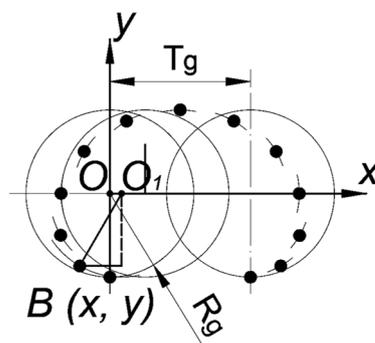
**Figure 3.** Calculation scheme for determining the deformable element's movement.
