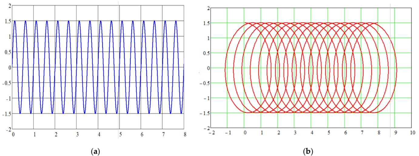
**Figure 4.** Microrelief profile with identical geometric parameters, according to Table 1: (a) sinusoidal profile; (b) rotary profile.
