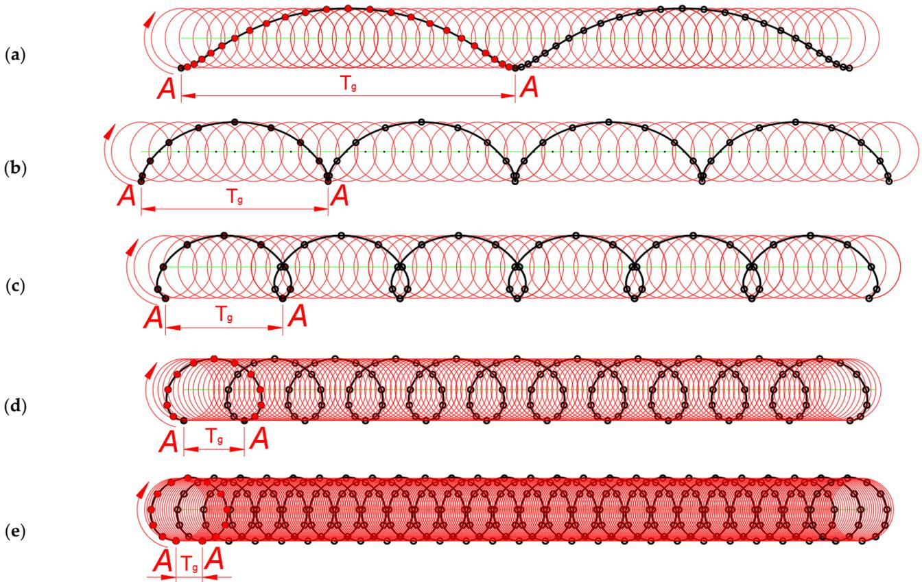
**Figure 1.** Transformation of the deforming element's trajectory when it rotates around a circle with radius  $R_g$  at different rotation rates. (a) shortened cycloid; (b) cycloid (c–e) elongated cycloids.
