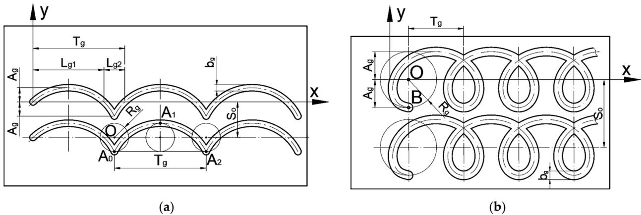
**Figure 2.** Basic geometric parameters of grooves and their location on a regular microrelief formed by rotation. (a) cycloid; (b) elongated cycloid.
