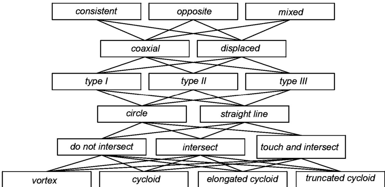
Figure 6. A set of variants of partially regular microrelief grooves formed by rotation.
