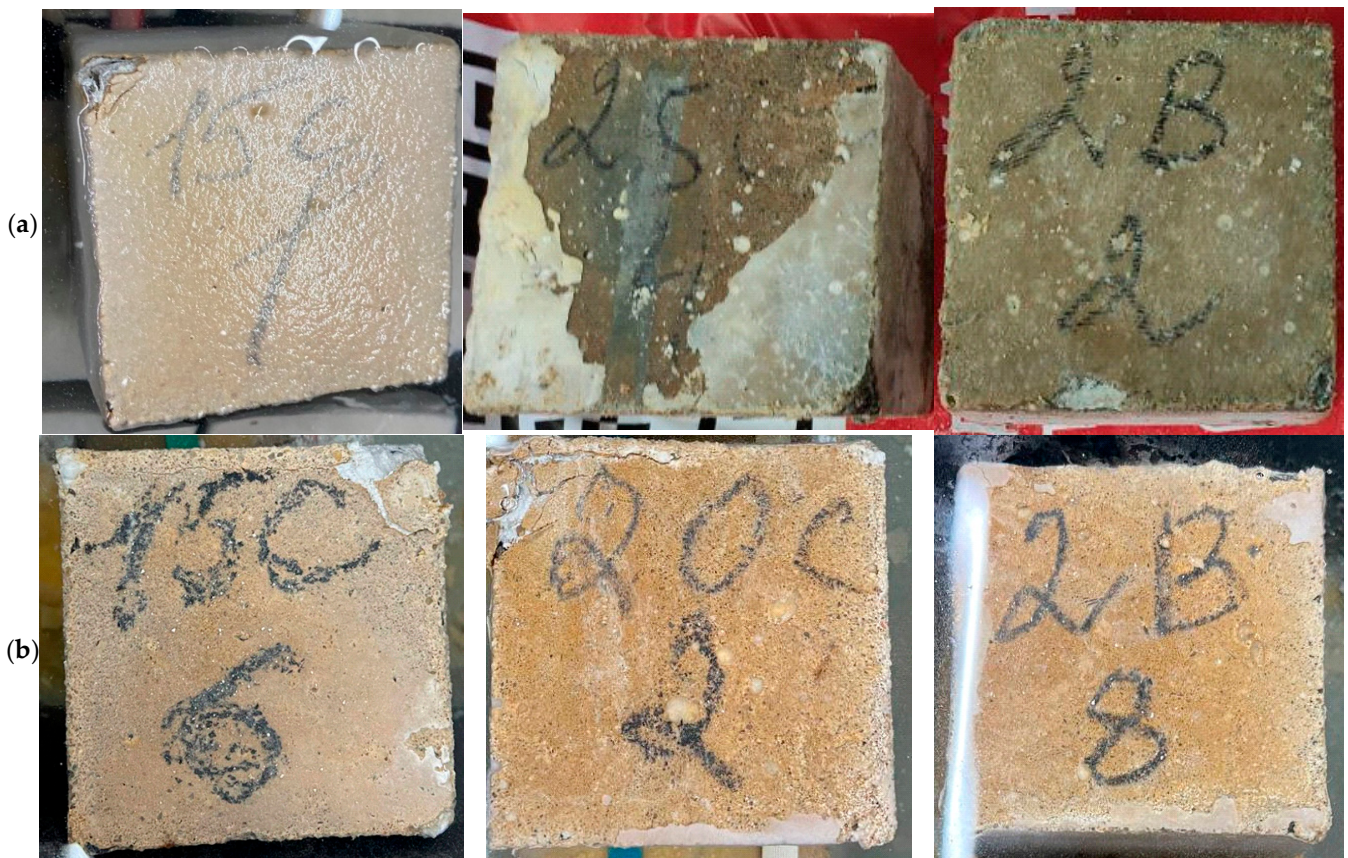
Figure 4. The appearance of the tested fiber concrete samples after 6 months (a) and 12 months (b) of aging in an acidic environment of pH = 3.
