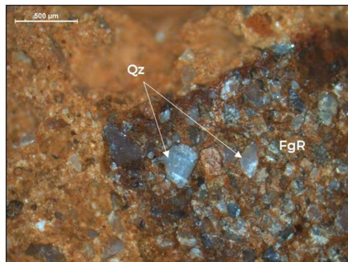
**Figure 35.** First-class brick sample composed of clasts of varying sizes, ranging from 60 to 7000  $\mu\text{m}$ , prominently featuring minerals and fragments of heterogeneous rock. The minerals are primarily
