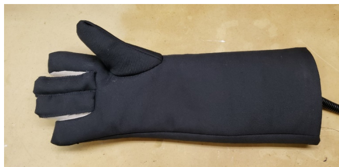
Figure 6. General construction of a prototype Active Textile glove with CNT inner liner. The glove has an outer protective layer, CNT center layer, and soft inner layer against the skin. The tube at the cuff is for air flow into the glove.
