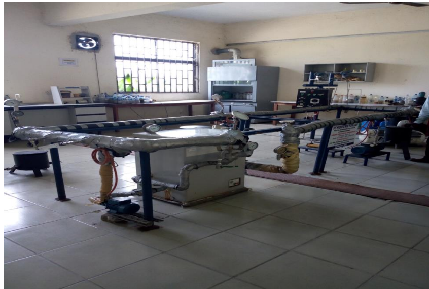
Scheme 1. Laboratory Mini Flow Loop for Hydrate Study.
