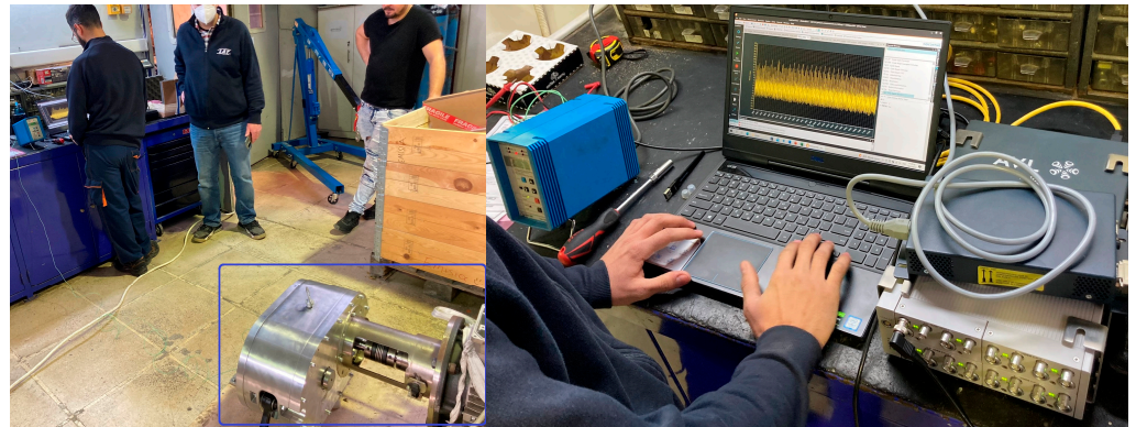
Figure 16. The final assembly of the rotary piston compressor and photographs from the experimental campaign.
