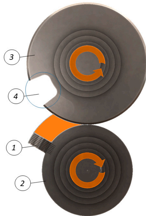
Figure 1. The piston-rotor position near the end of the compression process (some degrees before the primary peak pressure is developed).
