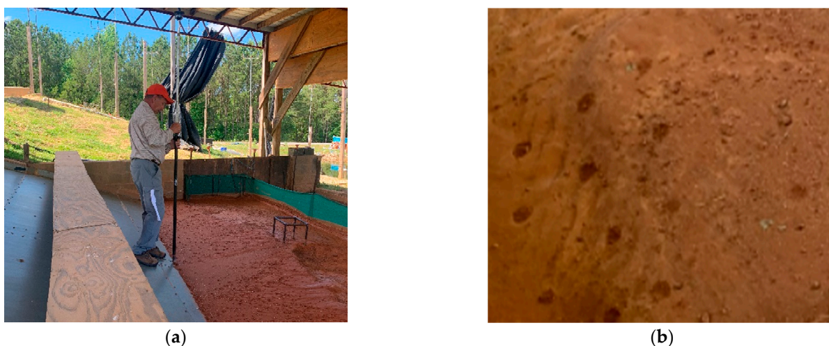
Figure 14. Challenges of using RTS to capture the surface: (a) A team member was holding the survey rod plumb; (b) “Dimples” on the soil surface created by the rod.
