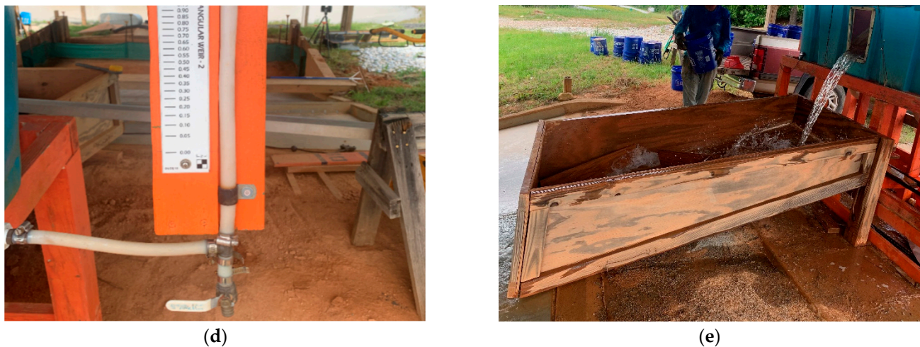
Figure 3. A full-scale erosion testing apparatus for this research study: (a) A full-scale testing apparatus; (b) Sediment collection area and silt fence; (c) Water tank connected to a pump; (d) Water flow gauge; (e) Soil and water mixing trough.
