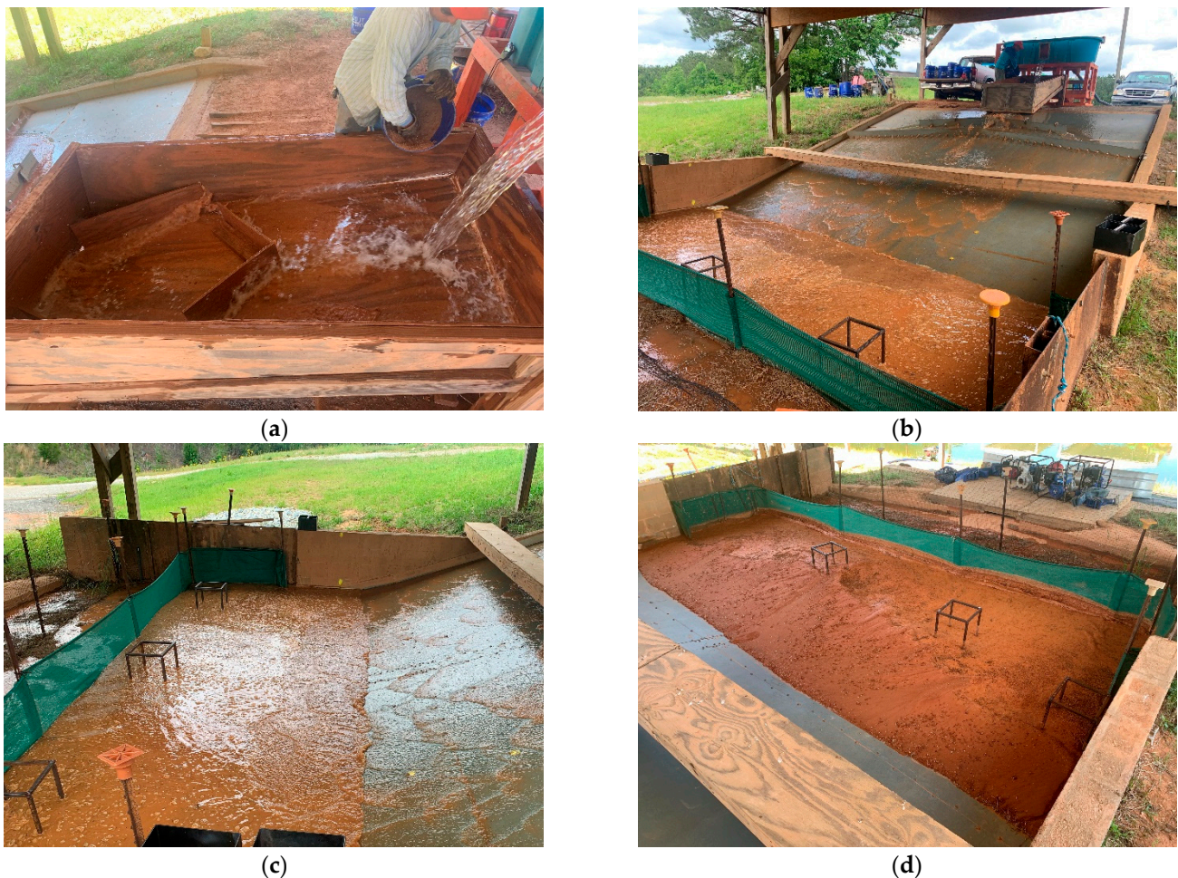
Figure 4. Erosion test in the full-scale apparatus: (a) Soil and water mixed in the trough at a constant rate; (b) Flow of sediment with water; (c) Mixture of water and soil accumulated in the testing area; (d) Drained testing area before measurements were taken.
