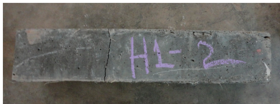
Figure 5. Beam specimen after flexural test.
