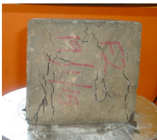
Figure 3. Specimens after compressive strength testing.
