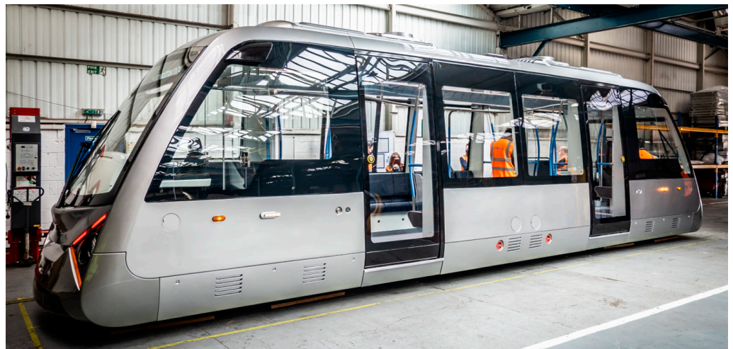
Figure 1. Coventry Very Light Rail (CVLR) demonstrator vehicle.
