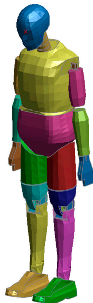
Figure 4. Hybrid-III (H-III) anthropometric test dummy.
