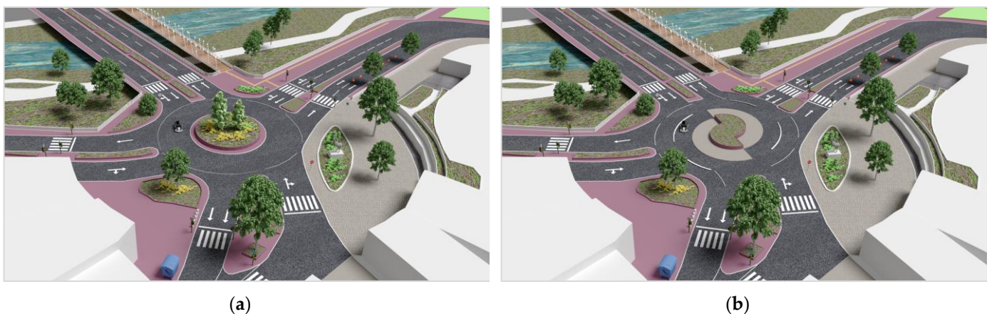
Figure 7. Before-and-after layouts of the examined roundabout. (a) Existing situation. (b) Virtual conversion into a turbo-roundabout [28].
