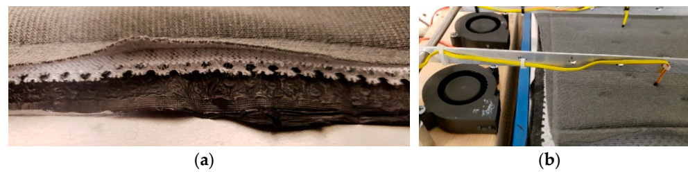
Figure 9. Glove composed nanofabric with four layers. (a) edge view of fabric, from top, 1-inner comfort layer to go against the skin, 2-spacer knit air insulation layer, 3-CNT heat spreading and shielding layer, and 4-outer waterproof layer. (b) Glove fabric on hot plate with two blower fans and two thermocouples. The inside surface layer of the fabric is in contact with the thermocouples. The outside surface layer of the fabric is in contact with the hot plate.
