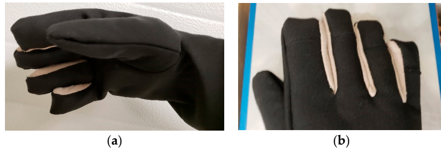
Figure 8. Nanoglove fabricated with a CNT inner layer that covers the full area of the glove. (a) Glove being worn. (b) Glove on hot plate for qualitative thermal testing. Thermocouples are moved to different locations in the glove. This glove has three fabric layers.
