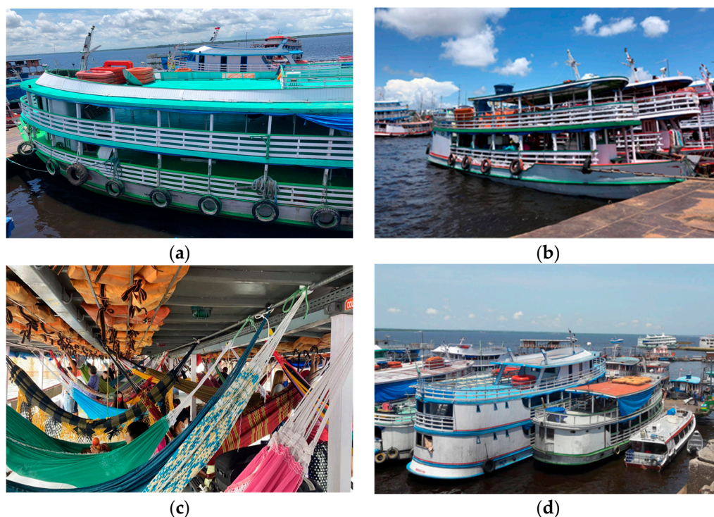
Figure 2. (a) Side of a gaiola vessel. (b) A complete view of a gaiola vessel in the port of Manaus. Credits: Daniel Bitencourt. (c) Typical hammock area arrangement in a gaiola vessel. (d) Porto de Manaus, nowadays. Figure credits: (a–c) Daniel Bitencourt, 2021; (d) [20].
