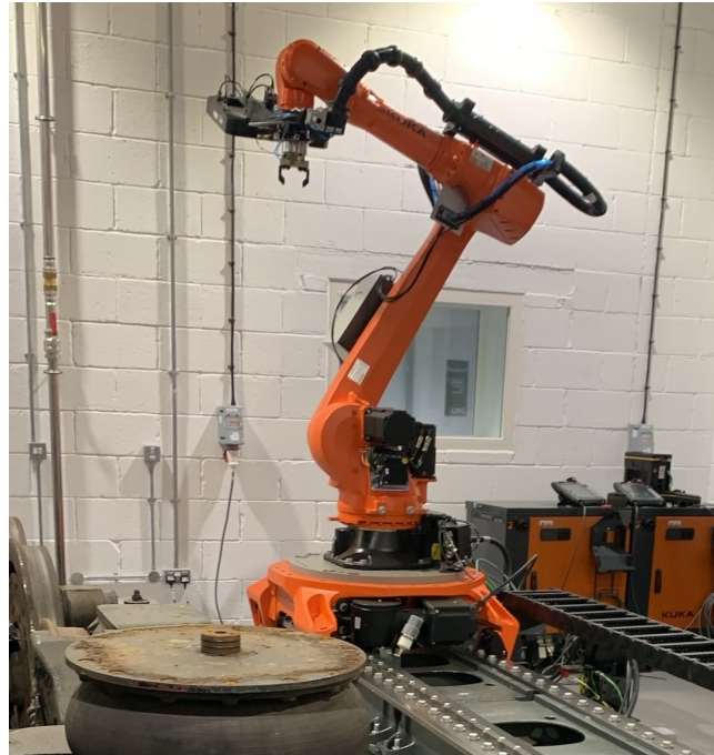
Figure 2. Robotic arm equipped with a high-resolution camera for automated image acquisition.
