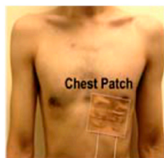
Figure 5. Two couplers constructed with the conductive textiles placed side by side on a human body [14].
