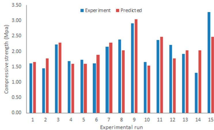
Figure 3. Comparison of experimental values with predicted values of compressive strength.
