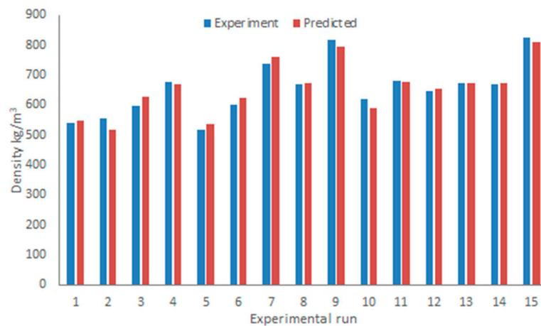
**Figure 9.** Comparison of experimental values of density with predicted values.
