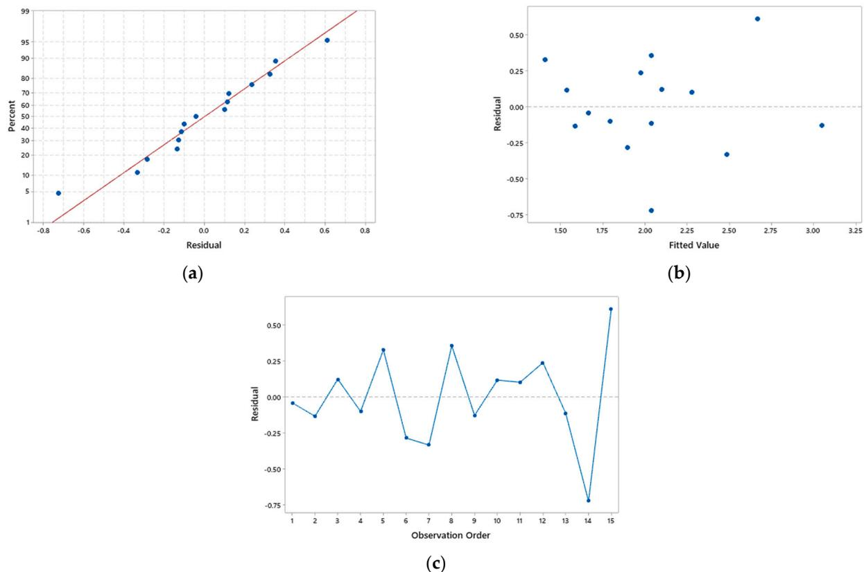
**Figure 2.** Plots to check assumptions of ANOVA for compressive strength: (a) normal probability plots; (b) residual versus fits; (c) residual versus observation order.
