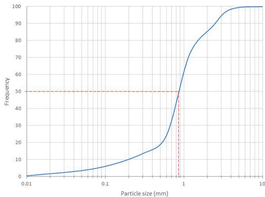
**Figure 1.** Particle size distribution of sawdust.
