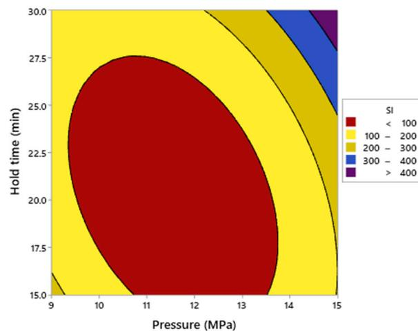
**Figure 7.** Contour plot of shatter index with pressure and hold time.
