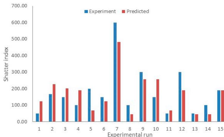
**Figure 6.** Comparison of experimental values of shatter index with predicted values.
