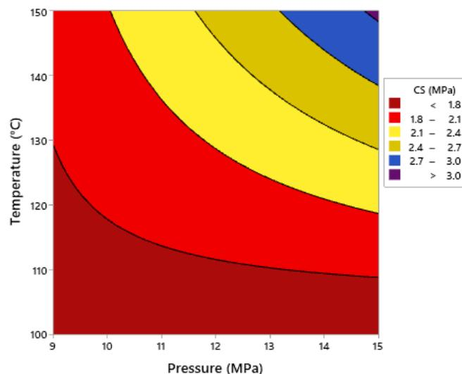
Figure 4. Contour plot of compressive strength with pressure and temperature.
