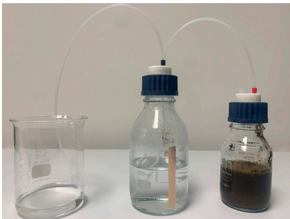
Figure 1. Picture representing the bioreactor. From right to left, the first bottle contains the inoculum mixed with the residual biomass to test; the second bottle is the water tank used to measure the quantity of biogas produced according to the volumetric method; and finally, the third bottle exclusively serves to avoid the dispersion of water ejected during the process.
