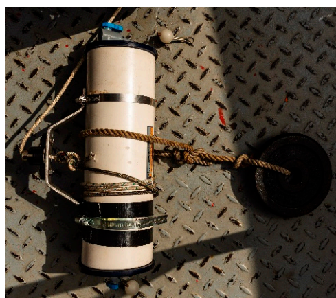
Figure 2. 2.2 L sampling tube from WILDSCO with added weight for faster sinking.
