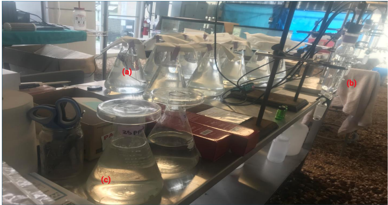
Experiment II mysid flasks. (a) eight mysid dosing flasks, (b) Artemia culturing setup, and (c) two extra water supply flasks; Marine Facilities Building, University of West Florida, Pensacola, Florida.
