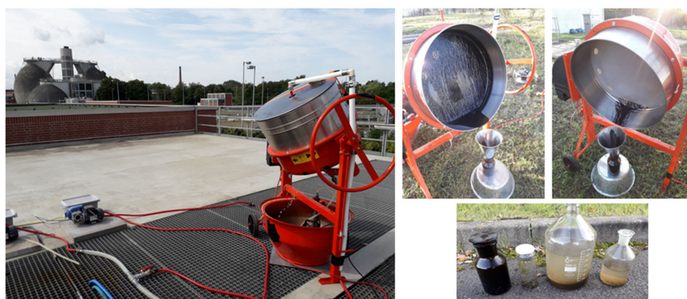
Figure 2. Field sample preparation process using the rotating sieve filter (RoSi) to concentrate the solids (>10 µm) for large-volume sampling.
