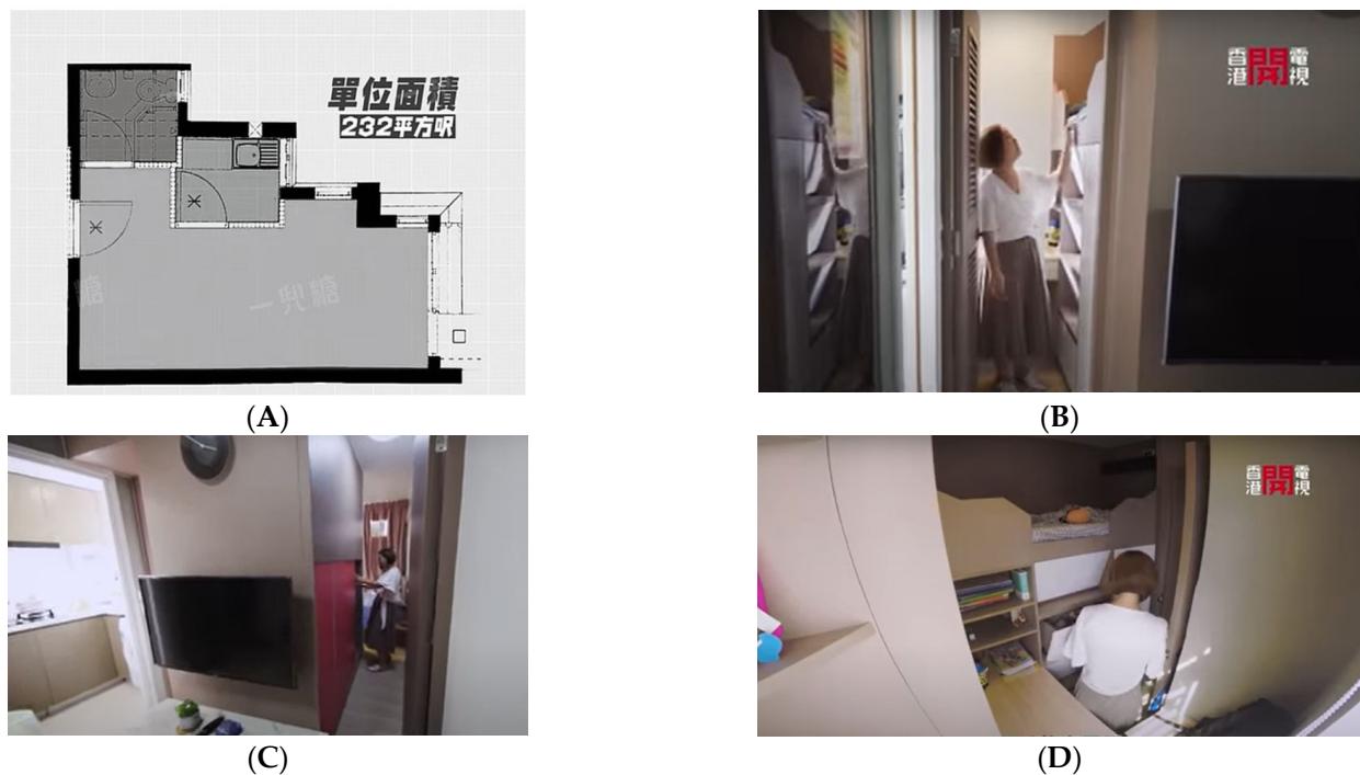
Figure 12. Furniture instead of wall partitions is used to separate public housing into different functional zones. (A) Layout of a 25 m 2 flat. (B) Use of two-sided wardrobe to separate bedroom spaces. (C) One side of the wardrobe and large bedroom. (D) Small bedroom with cupboard for children. Source: EP9-2 Interior Design of Small Units. Available online: https://www.youtube.com/watch?v=FaAXgq5iVqM . (accessed on 7 December 2023) [59].
