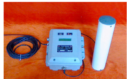
(b) KBD7 continuous electromagnetic radiation monitoring system
