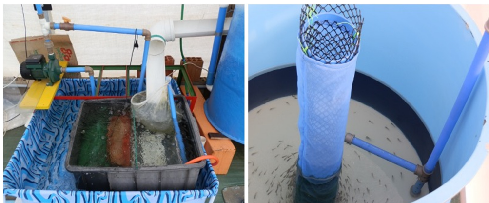
Figure 3. Panoramic view of the pump and pipes positioned vertically and horizontally in each tank to generate the water speed in the swimming exercise system in the larvae of Brycon amazonicus .
