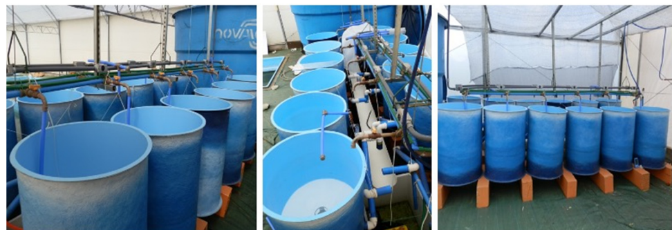
Figure 4. Schematic design of the experimental tanks and recirculation system (100-L tanks, water pump, mechanical and biological filters) that were used in the larvae swimming exercise protocol.
