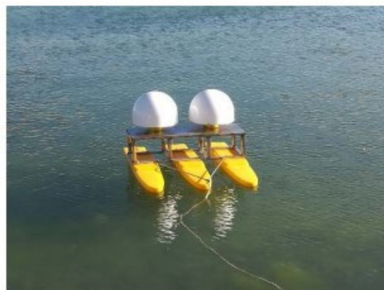
Figure 16. The GPSs mounted in a twinned trimaran plastic platform [20].
