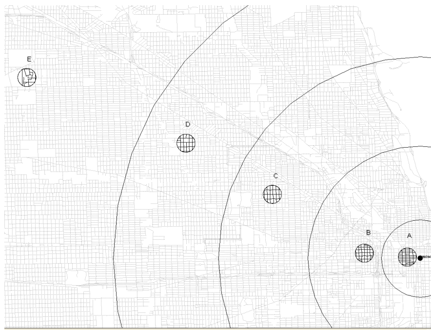
Figure 11. Region A, many alleys separate blocks: \text{dim} = 1.284 . Region B, a few alleys: \text{dim} = 1.258 . Region C, blocks, a bit larger: \text{dim} = 1.209 . Region D, blocks, a bit larger, along with more open space: \text{dim} = 1.198 . Region E, irregular patterns not uncommon with open space: \text{dim} = 1.181 .
