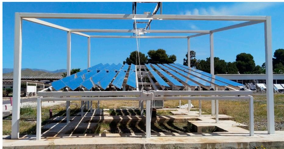
**Figure 2.** View of the prototype of LFC installed at the Plataforma Solar de Almería (Spain) during one of the tests to measure the flux of concentrated solar radiation in the focal plane.
