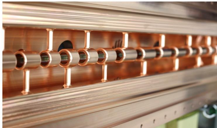
**Figure 4.** The fabricated center plate of the IH-DTL.
