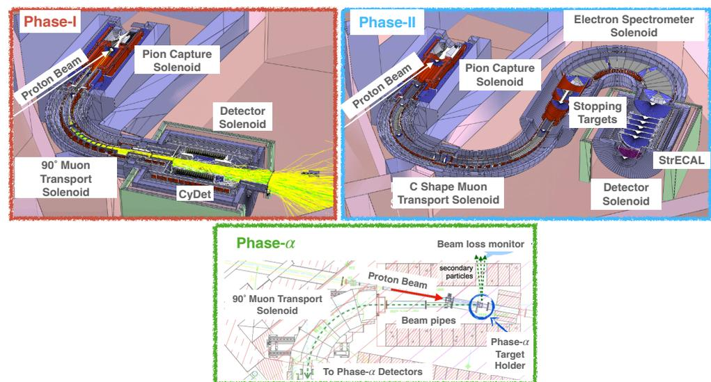
**Figure 1.** The COMET experiment is taking a phased approach with Phase-I (top left) and Phase-II (top right). An initial low-intensity beam run, Phase- $\alpha$  (bottom centre), will take place first.
