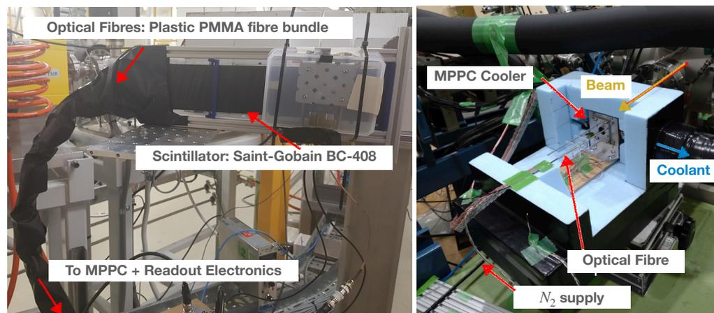
**Figure 2.** The CTH detector provides timing information for COMET Phase-I and utilises scintillator counters with MPPC photodetectors for photon readout. Recent progress includes preliminary beam tests with prototype counters using 100 MeV electrons at the Australian Synchrotron (**left**) and MPPC irradiation and cooling tests (**right**).
