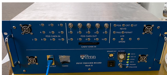
Figure 1. Front view of the Photon Trigger Board (University of Pennsylvania, Philadelphia, PA, USA), showing connectors in the chassis for some electronic subsystems: PDS, timing and LArTPC (NEVIS) trigger board.
