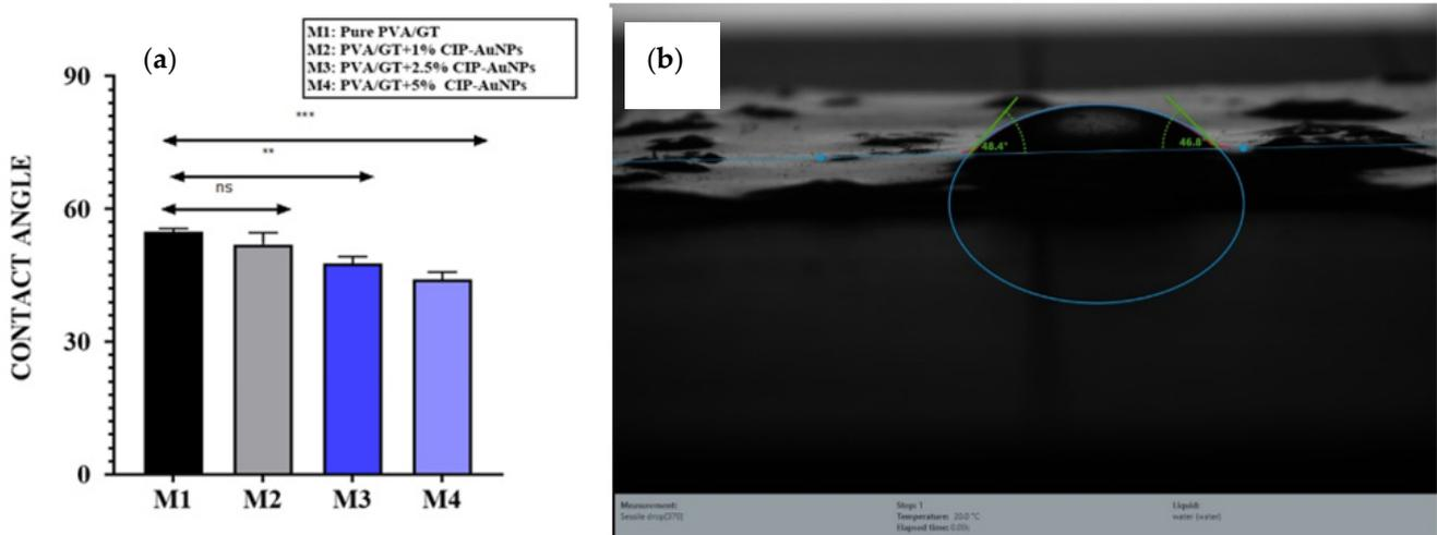
**Figure 3.** The contact angle of (a) pure PVA/GT, PVA/GT loaded with 1% CIP-AuNPs, PVA/GT loaded with 2.5% CIP-AuNPs, and PVA/GT loaded with 5% CIP-AuNPs. ns shows statistically insignificant results as the *p* value is greater than 0.005, while \*\*\* and \*\* shows statistically significant results as the *p* value is less than 0.005. (b) The contact angle of PVA/GT loaded with 5% CIP-AuNPs.
