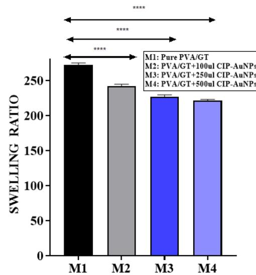
**Figure 2.** Swelling ratio of pure PVA/GT, PVA/GT loaded with 1% CIP-AuNPs, PVA/GT loaded with 2.5% CIP-AuNPs, PVA/GT and PVA/GT loaded with 5% CIP-AuNPs. \*\*\*\* shows statistically significant results as the *p* value is less than 0.005.
