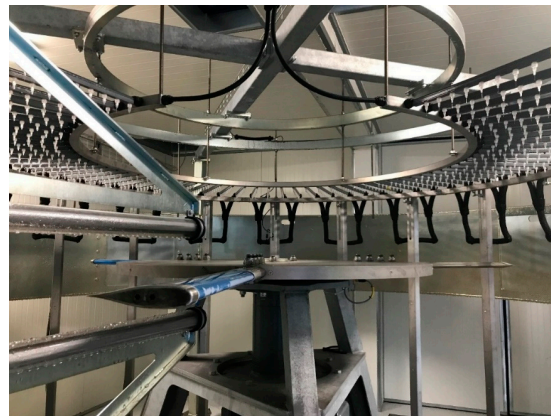
Figure 1. The R&D A/S whirling arm rain erosion tester at Offshore Renewable Energy (ORE) Catapult (Source: Offshore Renewable Energy Catapult).
