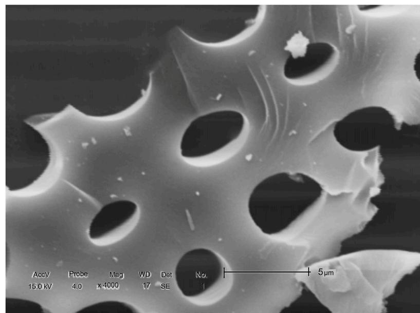
**Figure 6.** SEM detail of charcoal porosity.
