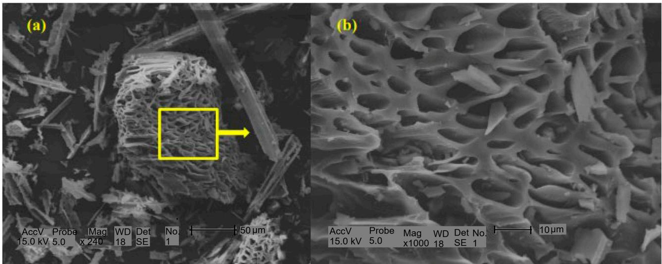
**Figure 5.** SEM of (a) charcoal and (b) SEM approximation of charcoal.
