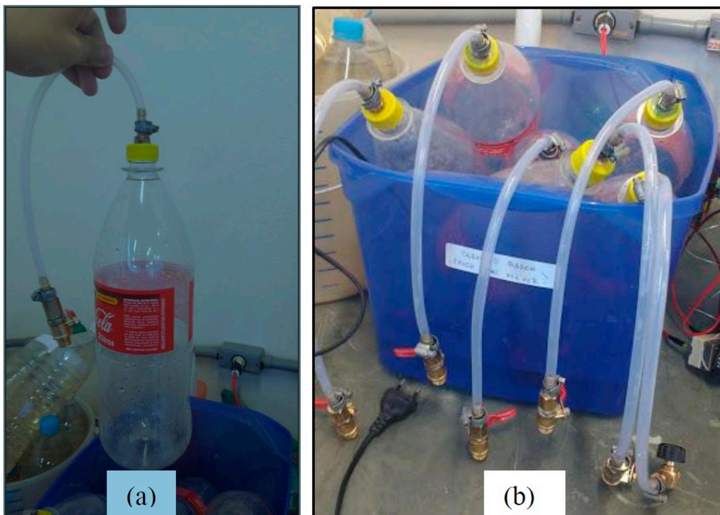
**Figure 1.** Experimental units: (a) bottle assembled (left); and (b) bottles immersed in the water system for heating (right).
