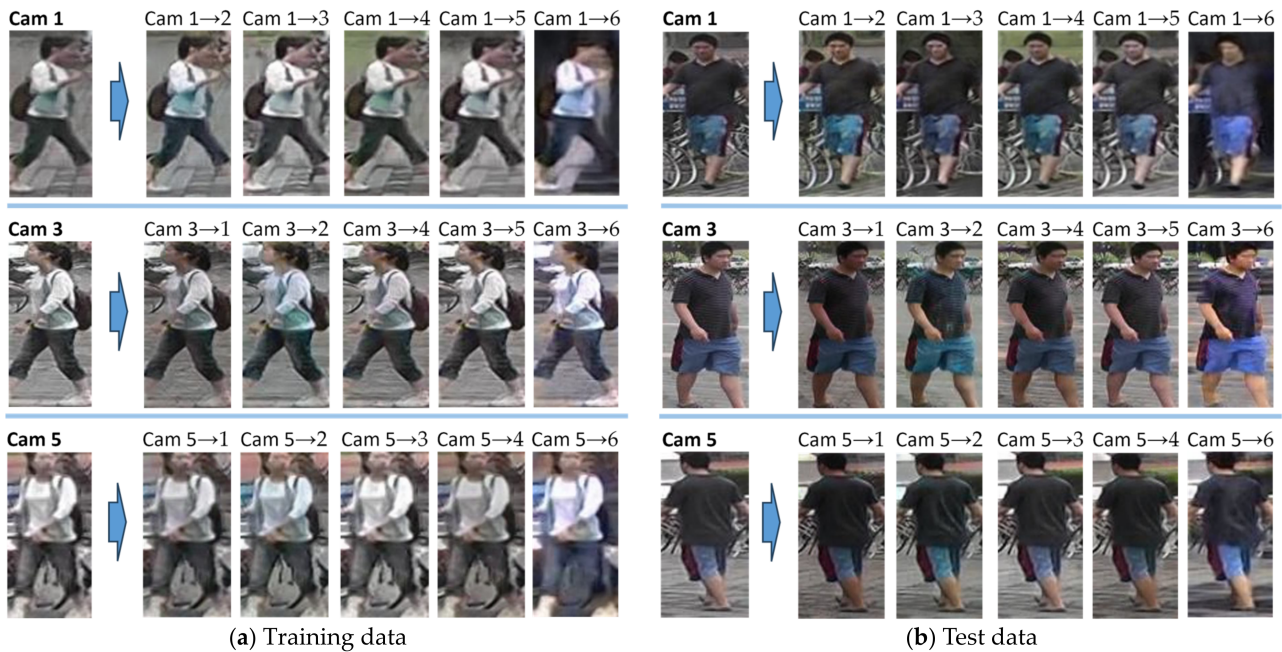
Figure 3. Some style-transferred samples in Market-1501 [39]. Each image, originally taken by a specific camera, is transformed to align with the styles of the other five cameras, both within the training and test data. The real images are shown on the left, while their corresponding style-transferred counterparts are shown on the right.
