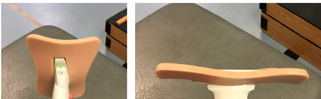
Figure 2. Custom-designed cast, housing a 10 cm ultrasound probe.
